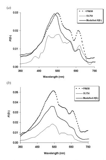
Figure 2. Comparisons of modelled R(0-) and measured (in water) R(0-) using OL-754 and PR-650 spectroradiometers for (*a*) St3 (Traid Bridge) and (*b*) St4 (Crookes Point).
